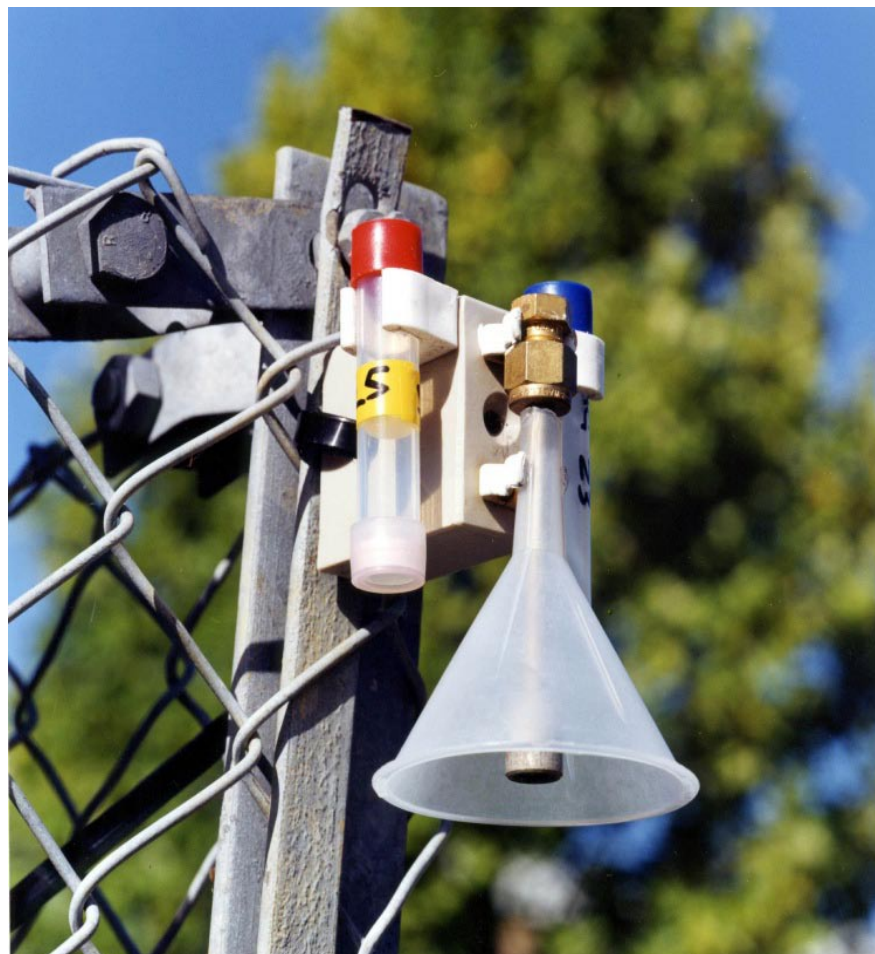
Fig. 8 Protective shelters and good mounting are essential in passive sampler surveys. Dietrich Schwela, WHO
